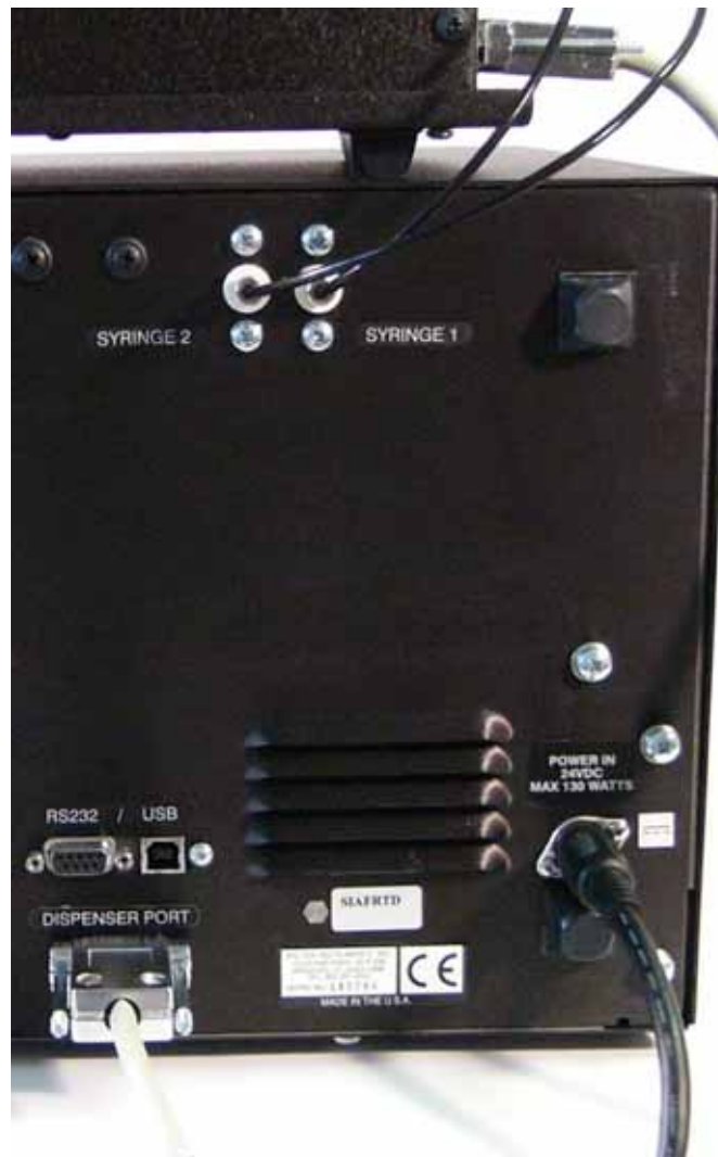
Figure 14: Dispense module connected to the reader (rear view)
