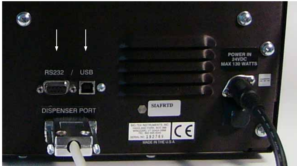
Figure 15: RS-232 serial and USB ports on the rear panel (injector model shown)
