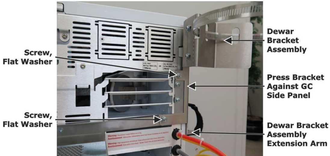
Figure 3-55 Dewar Bracket Installed to 8890 GC
