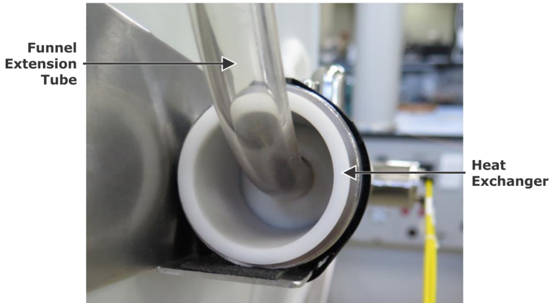
Figure 3-85 Extension Tube Inserted Into Heat Exchanger
