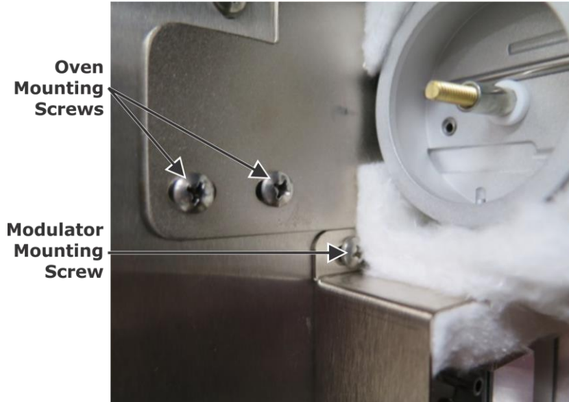
Figure 3-52 Mounting Screws for Modulator and Oven
