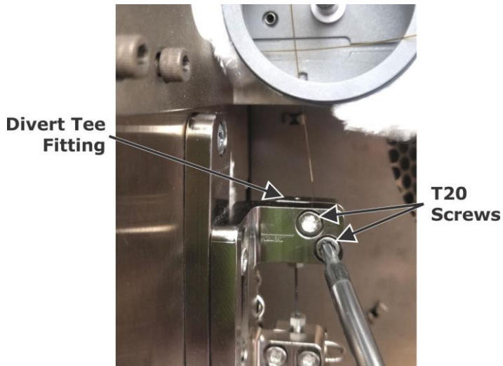
Figure 4-32 Loosening Screws on Divert Tee Fitting
