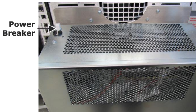
Figure 3-125 Control Box Power Breaker
