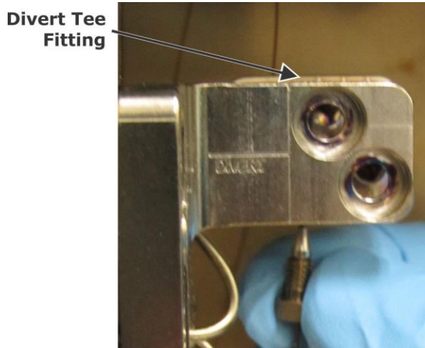
Figure 4-35 Inserting Nut and Ferrule into Divert Tee Fitting
