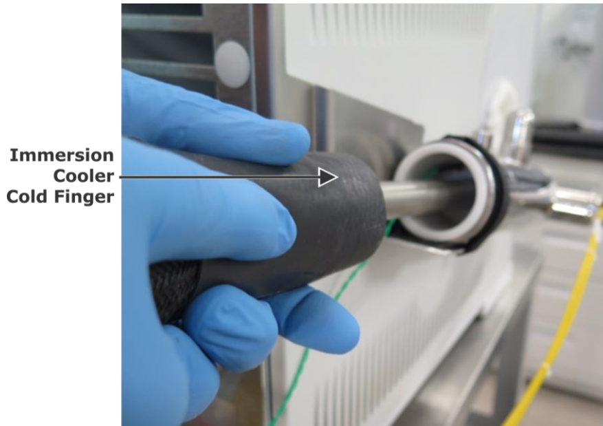
Figure 3-89 Inserting Immersion Chiller Cold Finger
