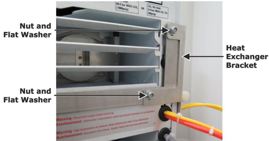
Figure 3-71 8890 CF Heat Exchanger Bracket Installed
