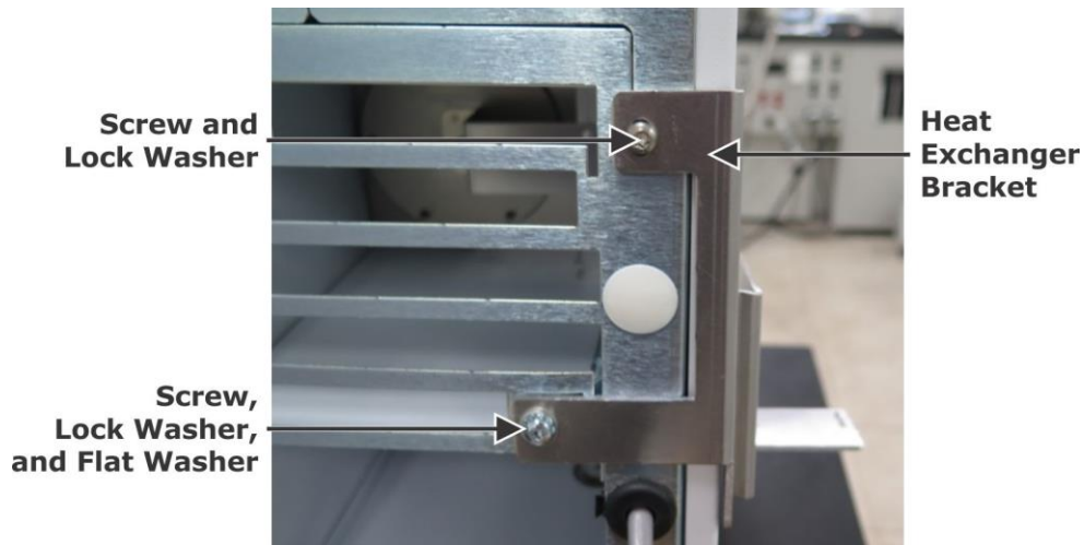
Figure 3-70 7890 CF Heat Exchanger Bracket Installed
