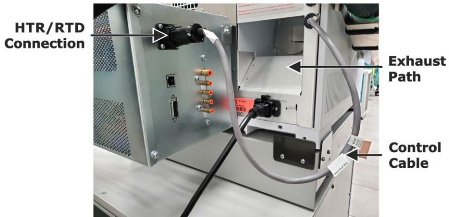
Figure 3-47 Control Cable Installed to 8890 Control Box
