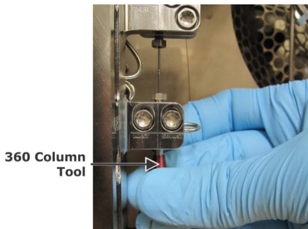
Figure 4-30 Removing 360 \mu\text{m} Nut and Ferrule from Primary Column
