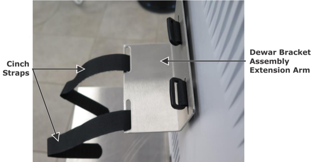
Figure 3-57s Inserting Strap through Bracket Extension Arm
