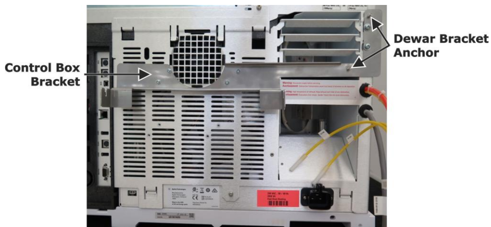
Figure 3-43 Modulation System Installation Locations on 8890 GC
