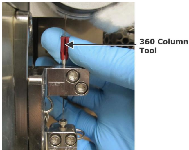
Figure 3-117 Using 360 Column Tool on Secondary Column
