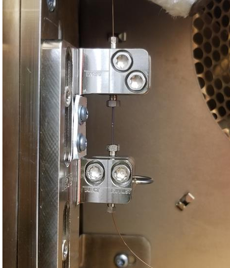
Figure 5-20 Flow Modulator Installed
