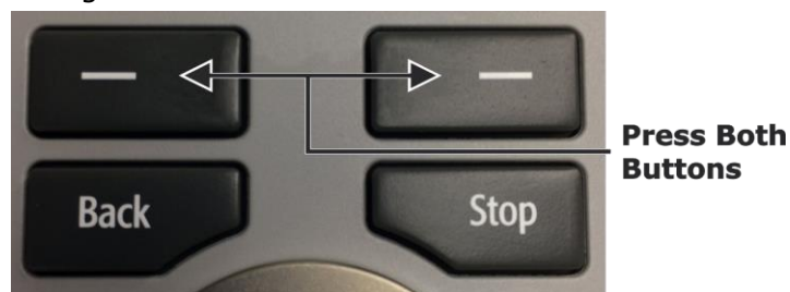
Figure 3-32 Extended User Level Access on PALterminal
