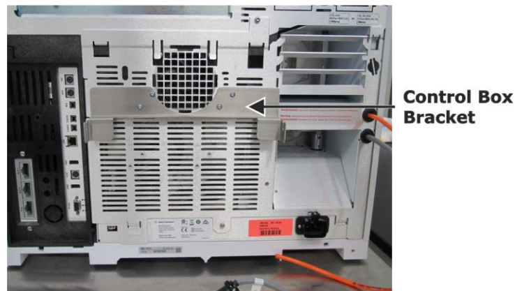
Figure 3-104 Control Box Bracket on 8890 GC
