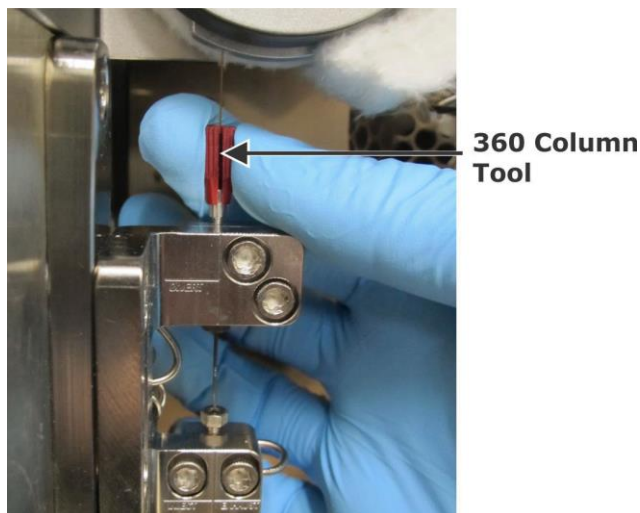
Figure 4-29 Removing 360 \mu\text{m} Nut and Ferrule from Secondary Column
