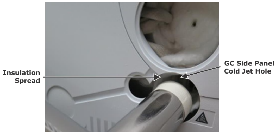
Figure 3-60 Insulation Spread for Cold Jet Insertion
