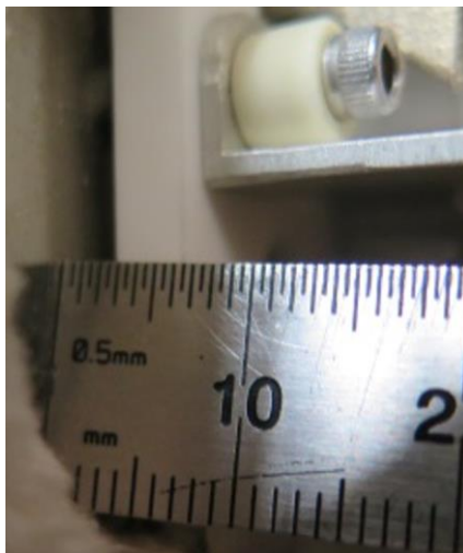
Figure 3-76 Measuring Gap Between Insulator and Heat Exchanger
