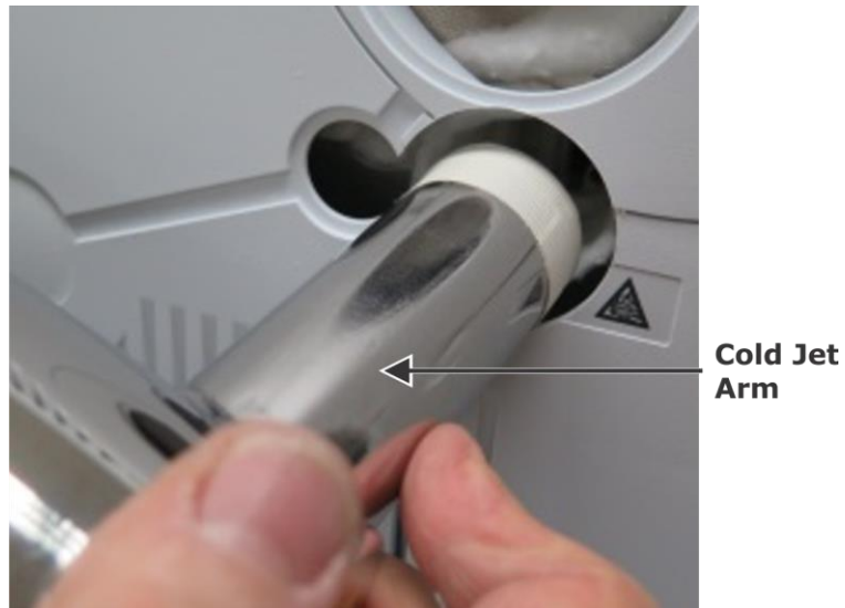
Figure 3-61 Inserting Cold Jet Arm into GC
