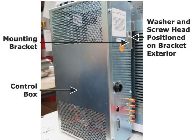
Figure 3-105 Control Box Installed to 7890 GC Mounting Bracket
