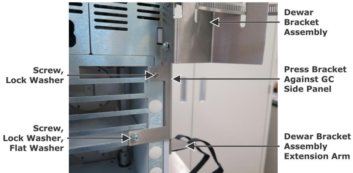
Figure 3-54 Dewar Bracket Installed to 7890 GC
