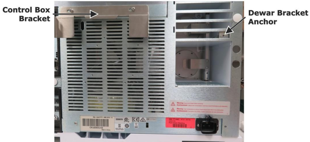
Figure 3-42 Modulation System Installation Locations on 7890 GC
