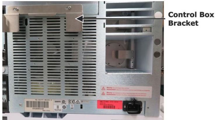
Figure 3-103 Control Box Bracket on 7890 GC
