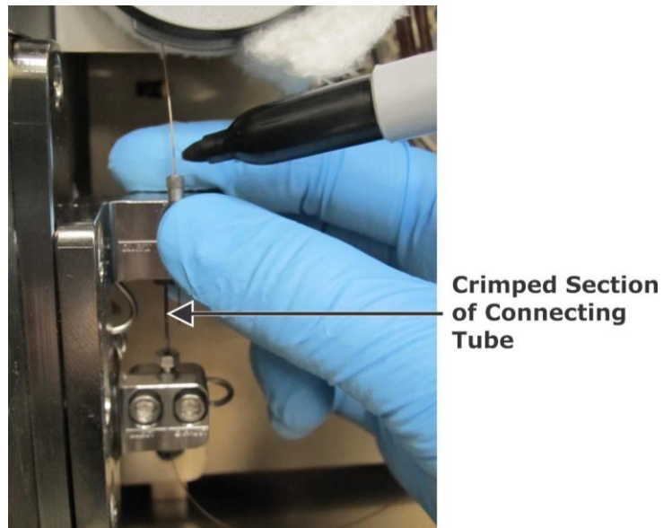
Figure 3-114 Marking Secondary Column Prior to Insertion
