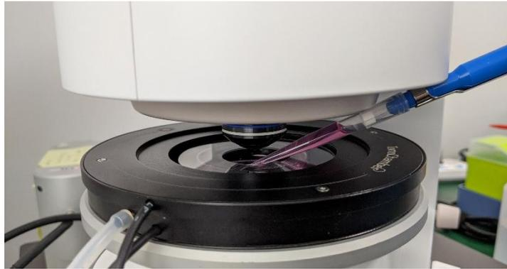
6. Click **[Working]** under **[Calibration]** tab to move the condenser lens to its previous working position. Carefully mount the lens-warmer on the condenser lens.
