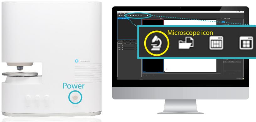
① Turn on the microscope by turning the knob clockwise. Power on 30 minutes before use to allow laser stabilization.
